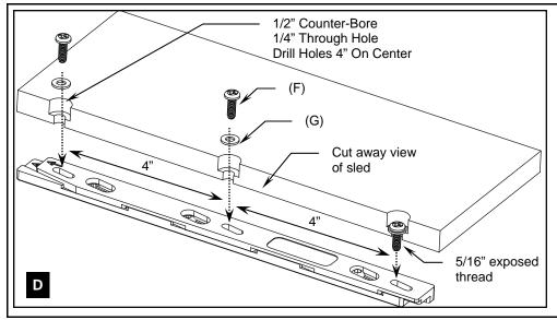
Depending on the size of your jig or fixture, a minimum of two mounting screws are required to mount the ZeroPlay<sup>™</sup> Guide Bar Assembly through the top of the jig or fixture.
